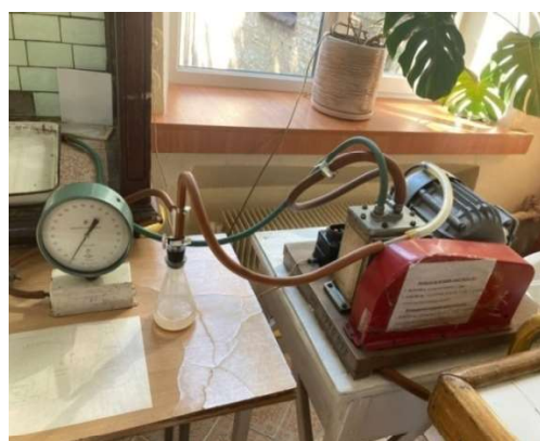
Fig. 3. Installation for vacuuming HNTs in electrolyte.
