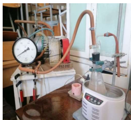
Fig. 3. Installation for vacuuming HNTs in electrolyte.
